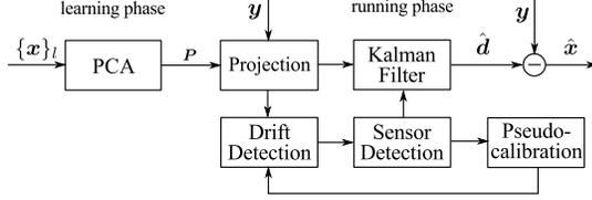
Fig. 1. SSP-KF Blind Drift Detection and Calibration Framework:  $\{\mathbf{x}\}_l$  is the measurement signal set in learning phase,  $\hat{\mathbf{d}}$  and  $\hat{\mathbf{x}}$  are estimated drift and calibrated signal
