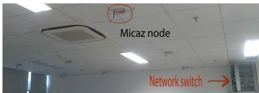
Figure 8. The actual picture of the test bed, inside the red circle is a Micaz node, and a network switch is used to connecting nodes to a server
