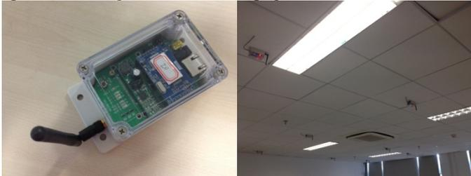
**Figure 2.** Left: Testbed node. Right: Testbed network installed on the ceiling of a lab room.
