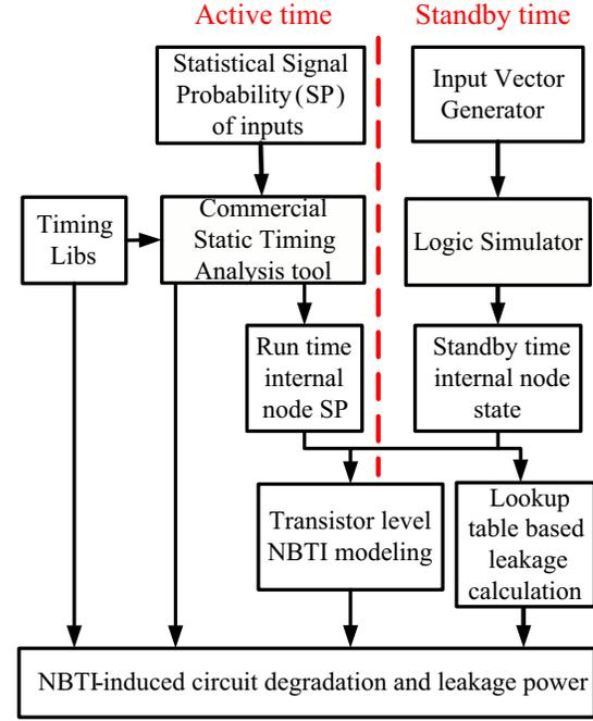
Fig. 6. Our NBTI/leakage analysis and optimization flow.
