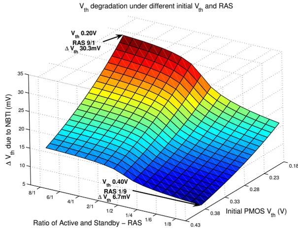
Fig. 8.  $V_{th}$  degradation comparison under different initial  $V_{th}$  and RAS.
