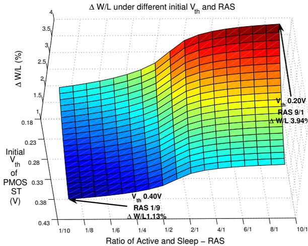
Fig. 9.  $\Delta(W/L)$  comparison under different initial  $V_{th}$  and RAS.
