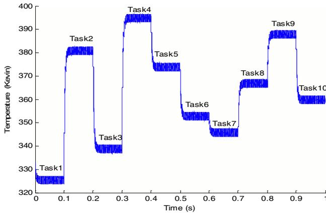
Fig. 2. Thermal profiles of running a task set on a typical processor.
