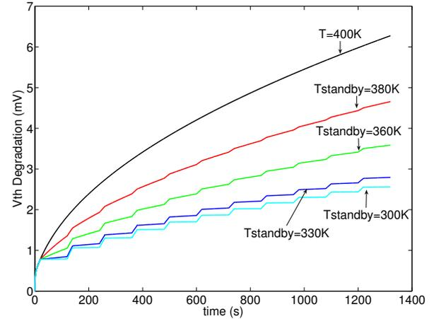
Fig. 4.  $V_{th}$  degradation with different  $T_{standby}$ . The active and standby time ratio RAS is set to be 1:5 and input signal probability is set to 0.5 in the active mode; in the standby mode, the input of PMOS is set to 0, which refers to the worst case  $V_{th}$  degradation.
