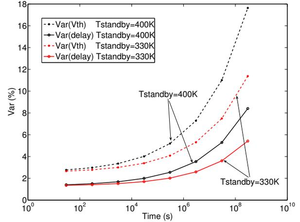
Fig. 5. Comparison between PMOS  $V_{th}$  degradation and C432 performance degradation.
