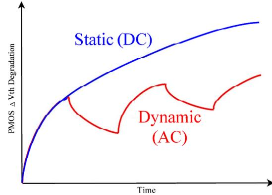
Fig. 1. The conceptual illustration of the PMOS  $\Delta V_{th}$  Degradation under DC and AC stress conditions, which shows the difference between static NBTI and dynamic NBTI.
