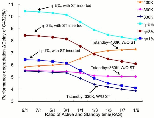
Fig. 11. Circuit degradation of C432 with ST insertion technique (three cases are the circuit without ST insertion under different  $T_{standby}$ ; the other three cases are the circuit with ST insertion under different Time0 timing constraint).
