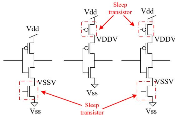
Fig. 10. Example of sleep transistor insertion on an inverter: footer, header, both footer and header.
