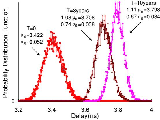
Fig. 12. Circuit performance distribution considering both variation and NBTI induced degradation (C880 in ISCAS85 benchmarks).
