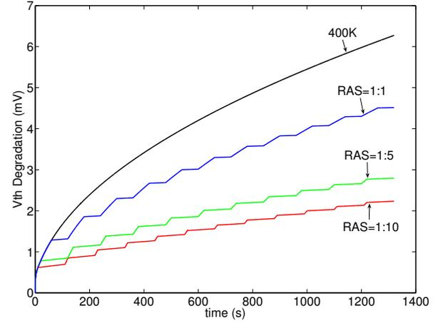
Fig. 3.  $V_{th}$  degradation with different active and standby time ratio (RAS).  $T_{active} = 400K$ , the input signal probability is set to 0.5 in the active mode; in the standby mode, the input of PMOS is set to 0, which refers to the worst case  $V_{th}$  degradation.
